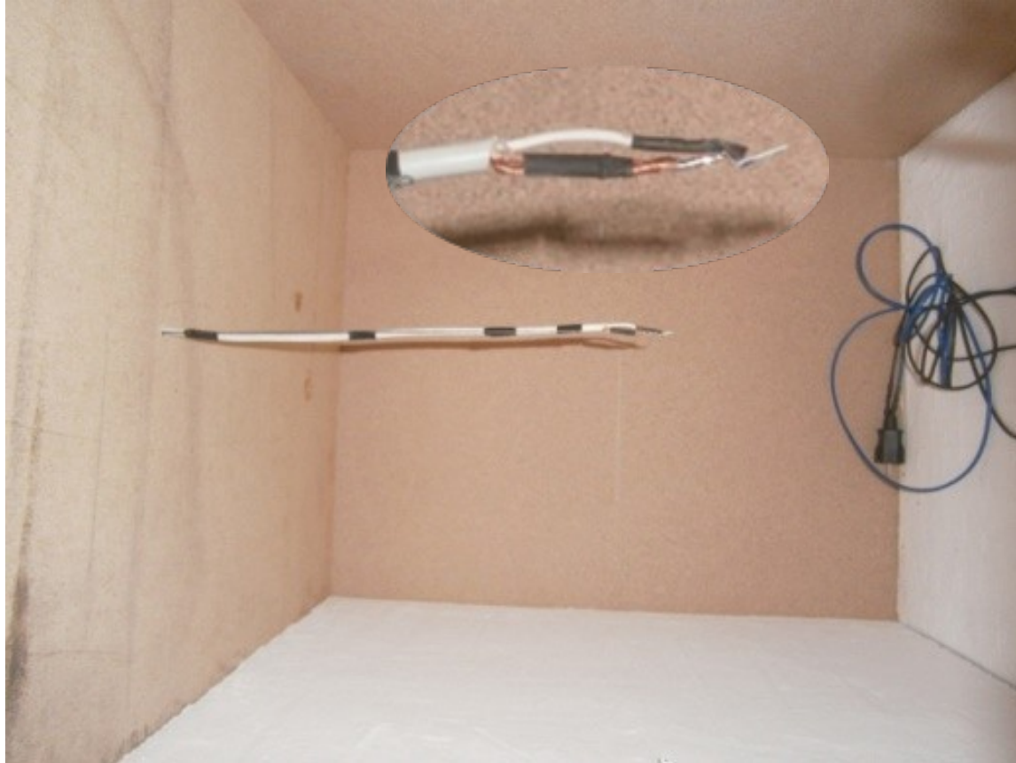
Figure 6. The interior of the test model – show the position of the PT100 probe
