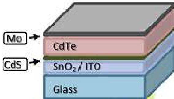
**Fig. 2.** *Solar cell device based on CdTe*
