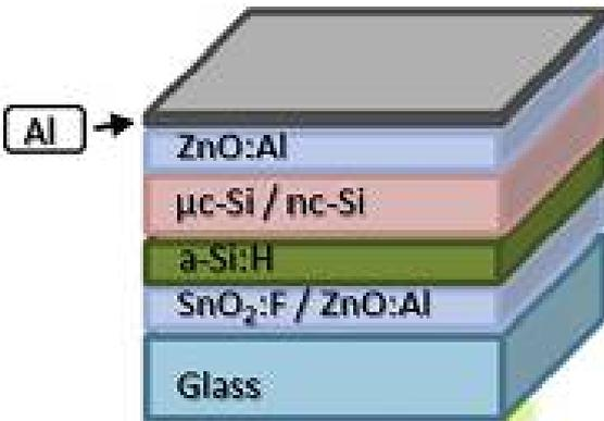
**Fig.** *Solar cell device based on a-Si/ $\mu$ -Si*
