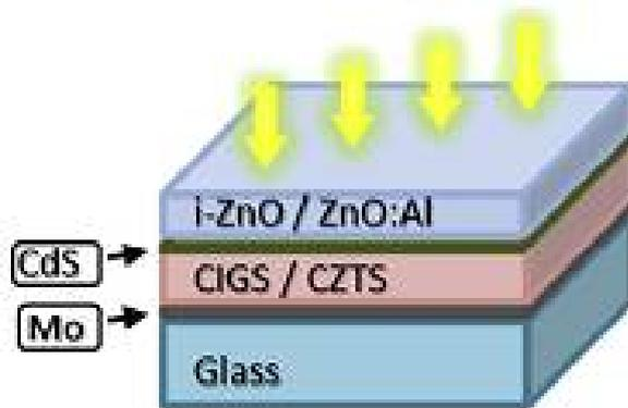
CIGS is the only commercial TF technology that has continually reported efficiency improvements of its record cells during the last decade, with efficiency at present of 13 % for modules and 20 % for cell.
